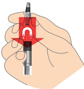
The bits can be inserted in all adapters with magnetic and will be locked into the adapters automatically.
