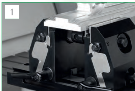
Clamped workpiece using jaw plates with pins. The high tractive force creates a positive clamping situation.
