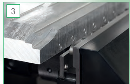
Blank after clamping. Clamping pin imprint is visible on the edge of the workpiece.
