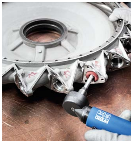
Surface finishing of a diffuser with POLINOX cross buffs PNST and conical tungsten carbide burrs with radius end.
