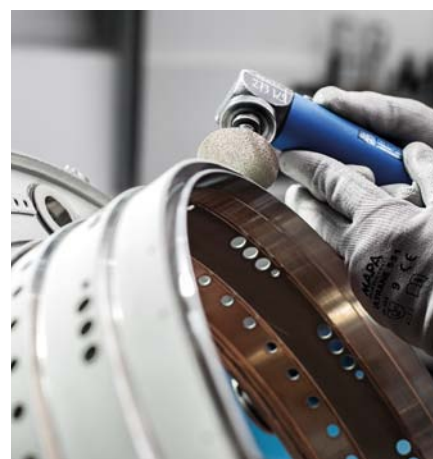
Removal of coatings with a COMBIDISC diamond abrasive disc.
