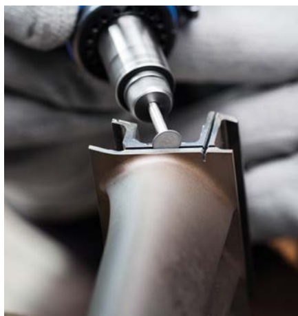
Cleaning and machining slots with a diamond grinding point.
