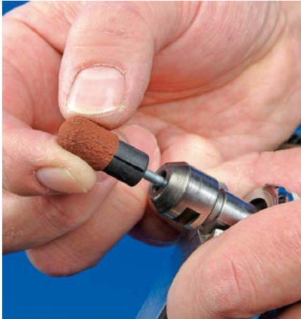
Weld dressing of radii on inner edges with POLICAP abrasive caps, types A, CO-COOL and SiC-COOL.
