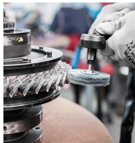
Deburring work on a rotor with wheel brushes of type SiC.
