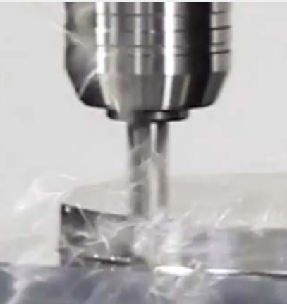
▲ Rough Cutting Ultra-micrograin carbide supplies the rigidity to keep the chips flying. Highly polished 3-flute design ensures they'll keep flying – cut after cut.
