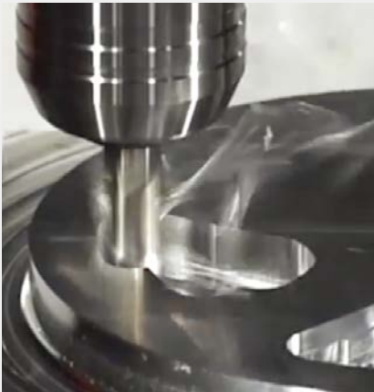
▲ Ramping In steep, aggressive ramping conditions, the ALU-POWER HPC holds its own to resist the torsional stress from extreme helical output.
